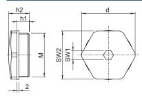
$\begin{array}{ll} \text{M = Thread size} & \text{d = Width across corners} \\ \text{h1 = Thread length} & \text{h2 = Dimension h2} \\ \text{SW1 = Width across flats hexagon socket} \\ \text{SW2 = Width across flats} \end{array}$
